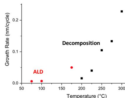
The H<sub>2</sub> plasma co-reagent enables deposition at lower temperatures down to 75°C, which is 100°C lower than thermal decomposition. This allowed films to be deposited on Melinex™ plastic, glass, titanium nitride and silicon.
