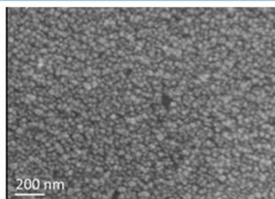
To explore the nano-scale morphology a holey carbon grid was coated using the same conditions and examined using transmission electron microscopy. At a magnification of 250k atomic lattice imaging the copper crystallites exhibit twinning.
