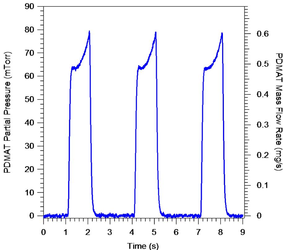
Carrier Gas Flow Rate: 1 slm
