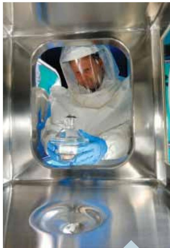
**Figure 2:** Specialised containment equipment is used for handling HPAPIs
