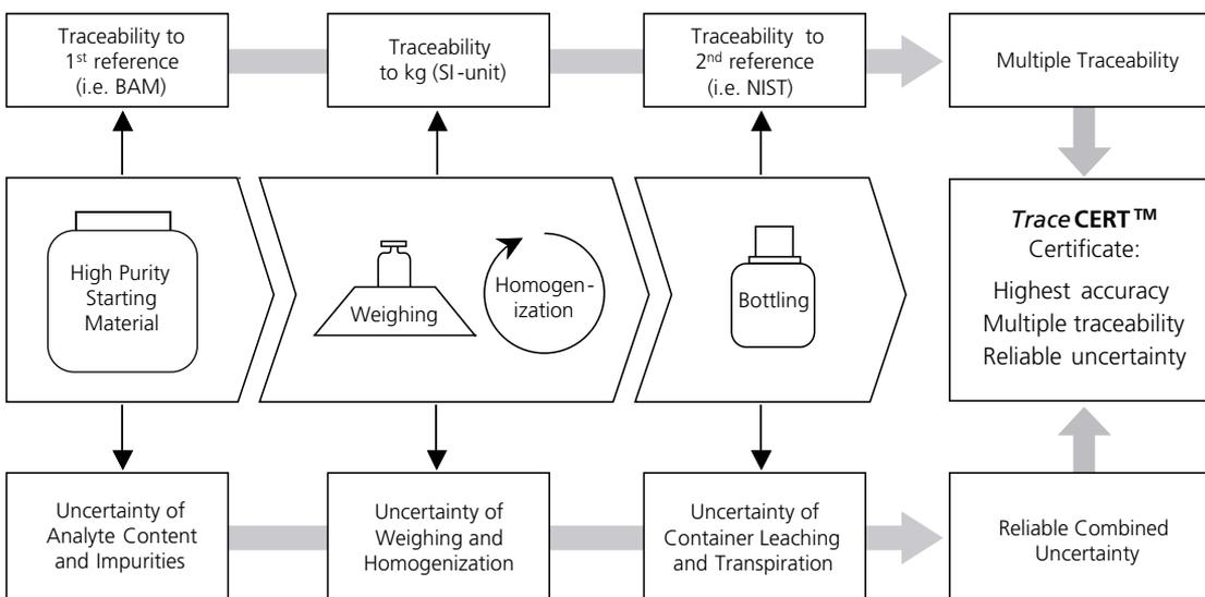
**Figure 1** ..... Schematic representation of the production design and certification of Sigma-Aldrich *TraceCERT™* products. This approach was established for the preparation of intercomparison samples at the highest metrological stage.
