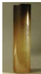
Figure 2. Typical Bridgman grown PMN-PT crystal (diam. = 1.8 cm)
