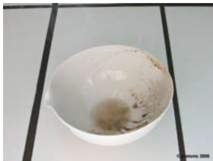
Treatment of tributylmethylphosphonium dibutylphosphate by a gas burner flame for 60 seconds.
