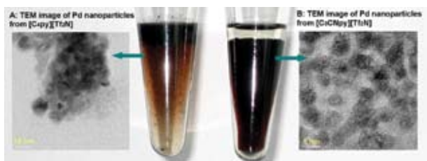
Figure 1: Comparison of ionic liquid-organic biphases after catalysis and TEM images of nanoparticles extracted from the ionic liquid phase; (left) [C_2py][Tf_2N] and (right) [C_3CNpy][Tf_2N] . Note the absence of precipitates and clarity of the organic phase with the nitrile-functionalized ionic liquid.
