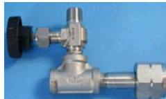
Figure 10. CGA 350 outlet adapter assembled with a flushing tee and 1/4 inch needle valve
