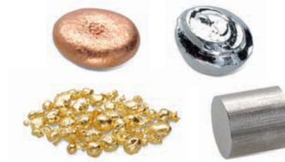
Figure 2 Only well-characterised and high-purity starting materials are used for TraceCERT calibration standards (clockwise from upper left: copper, zinc, nickel and gold).
