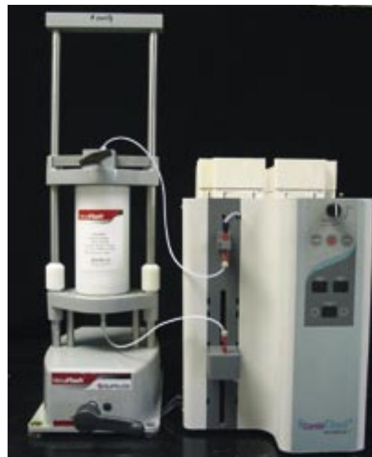
Figure 2 ..... Using the VersaFlash® Station to connect large volume VersaPak® cartridge to an Isco CombiFlash® system. The same design can connect VersaPak® to any flash system.
