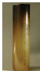
Figure 2. Typical Bridgman grown PMN-PT crystal (diam. = 1.8 cm)
