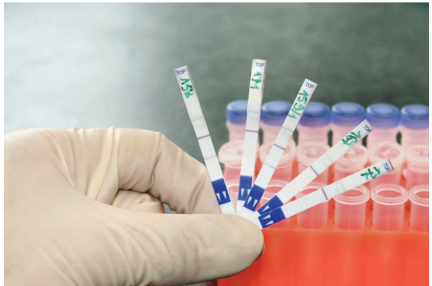
Figure 1: Borrelia lateral flow assay (Analytik Jena)
