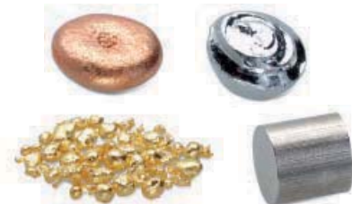
Figure 2 Only well-characterized and high-purity starting materials are used for TraceCERT calibration standards (clockwise from upper left: copper, zinc, nickel and gold).
