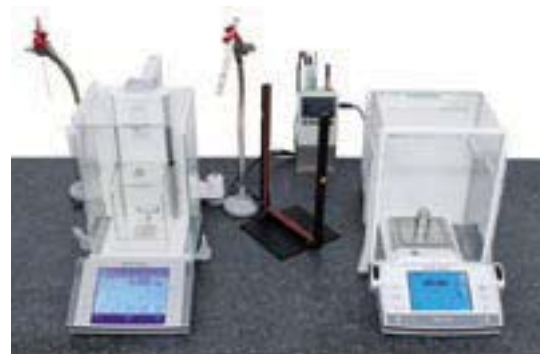
Figure 2 ..... High precision balances on a 1,000 kg granite weighing table with static discharge unit and climate monitoring instrument for air buoyancy correction
