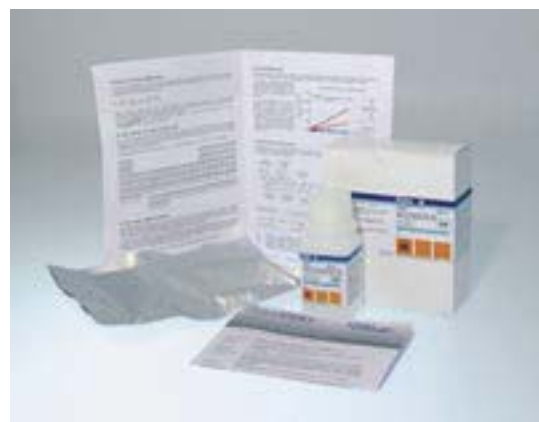
Figure 6 ..... Packaging of TraceCERT TM Ultra standards for ICP to ensure \pm 0.2\% expanded uncertainty for the certified value. Only when using specially selected Al-coated bags the specifications of the CRM can be guaranteed to have a shelf life of up to 4 years
