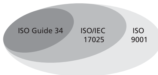
Figure 1 When climbing up the “quality ladder,” only with ISO Guide 34 (in combination with ISO/IEC 17025) can CRM producers achieve the highest level of reliability.
