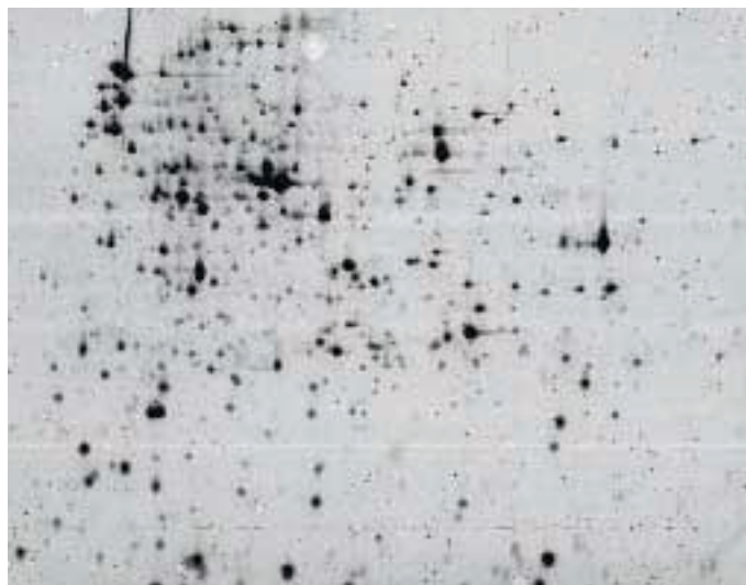
Figure 2: 2-D Electrophoresis of E. coli proteome. First dimension was performed on pH 3-10 gradient strip. Staining was performed using Ruthenium II tris (bathophenanthroline disulfonate). Courtesy of Andreas Lamanda, University Bern
