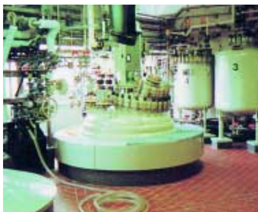
Figure 5: First floor of the production plant with distilling retort and several receivers to collect the different fractions.
