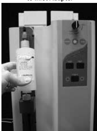
Figure B. Attaching Cartridge to Inlet Adapter
