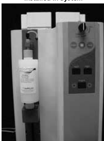
Figure C. Cartridge Installed in System
