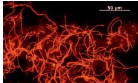
Figure 2 Fluorescence-marked Microthrix parvicella in activated sludge; Source: © Bayerisches Landesamt für Umwelt
