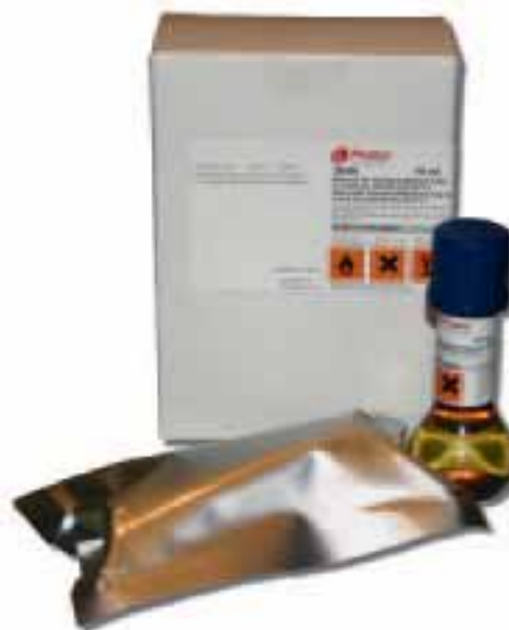
Figure 2 Mineral oil CRM with optimized packaging. The label carries the certified value, measurement uncertainty and expiration date.
