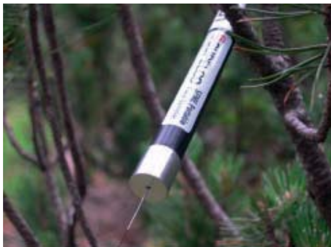
Figure 2 An SPME Fibre with Carboxen/Polydimethylsiloxane (75 µm) Stationary Phase Captures Both Non-Polar and Medium Polarity Volatile Metabolites Released from Plants
