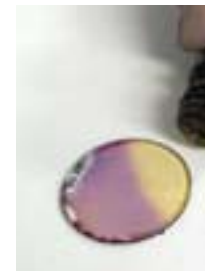
Figure 3 ..... Differential color change on an optical sensor disk upon deposition of analyte solution
