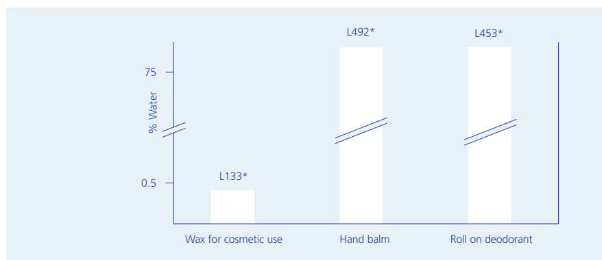
Figure 1 ..... Moisture levels of some cosmetic products determined using HYDRANAL®-reagents. (Note: * Laboratory Reports)
