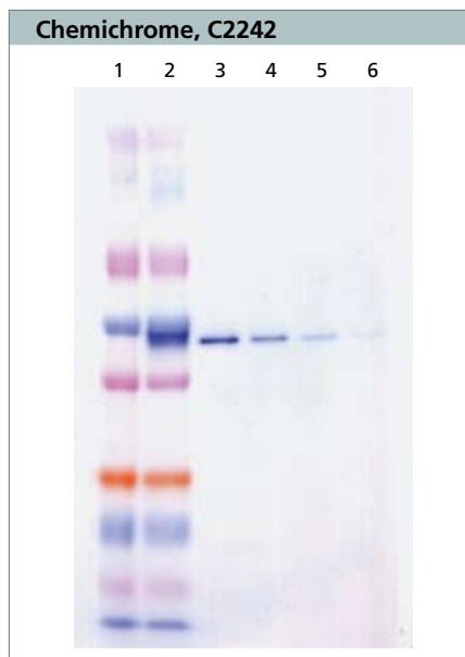
ColorBurst (lane 1), Chemichrome (lane 2), and FLAG®-BAP concentrations of 80 ng, 40 ng, 20 ng and 10 ng (lanes 3-6, respectively) were run on a 6-15% Tris-Acetate gel, transferred to PVDF and developed with a TMB substrate (T0565).
