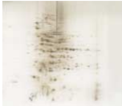
4 \mu g of E. coli whole cell extract was separated by IEF using a ProteoGel™ IPG strip (pH 3-10) ( L2531 ), equilibrated using ProteoGel IPG Equilibration Buffer ( L7281 ), and run on a Tris-Acetate 2D 8-18% gel. Following electrophoresis, the gel was stained with ProteoSilver ( PROT-SIL1 ).
