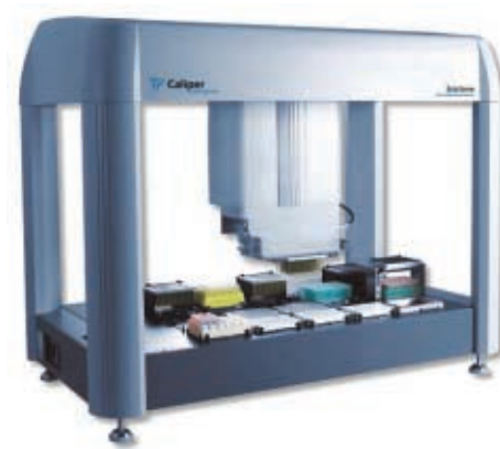
Figure 1. Sciclone ALH 3000 Liquid Handling Workstation. The automated ELISA method utilizing the ANTI-FLAG HS M2. Coated plates was developed and validated for the Sciclone ALH 3000. The system used in these experiments was configured with 96-Channel. High Volume Head, Z8™ Pipettor, Gripper, and a Bulk Dispense Module with syringe pump.
