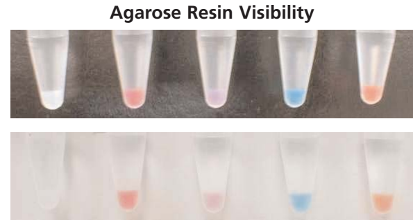
Fig. 2. Dyes covalently attached to agarose make agarose pellets more visible. The same samples were photographed with a black background (upper panel) and a white background (lower panel) to illustrate relative contrast.
