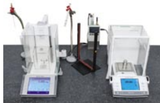
Figure 2 ..... High precision balances on a 1,000 kg granite weighing table with static discharge unit and climate monitoring instrument for air buoyancy correction
