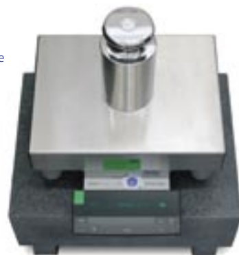
Figure 2 ..... High precision balances on a 1,000 kg granite weighing table with static discharge unit and climate monitoring instrument for air buoyancy correction
