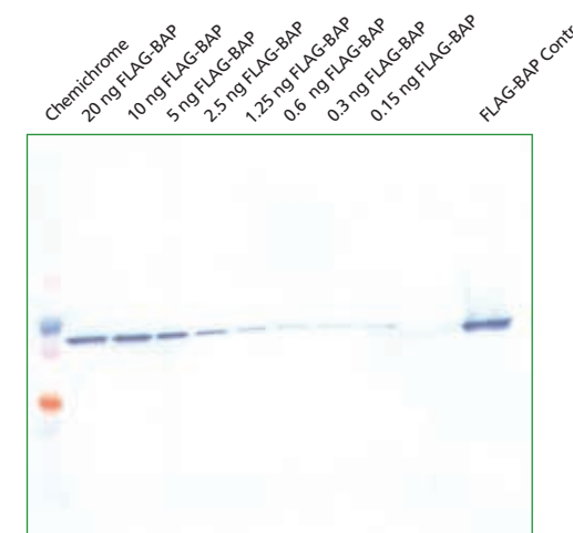
Sigma PVDF membrane (0.15 ng sensitivity) The FLAG® BAP control was used to show how a typical Western blot would be performed with a control. 20 to 0.15 ng of FLAG-BAP was detected on PVDF. No other bands besides FLAG-BAP and Chemichrome IgG (heavy chain) band were detected.
