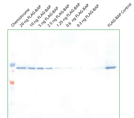
Sigma nitrocellulose membrane (0.3 ng sensitivity) The FLAG-BAP control was used to show how a typical Western blot would be performed with a control. 20 to 0.3 ng of FLAG-BAP was detected on nitrocellulose. No other bands besides FLAG-BAP and Chemichrome IgG (heavy chain) band were detected.
