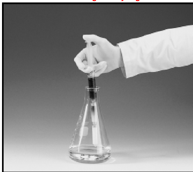
Figure A. Adsorbing Ethidium Bromide on Rezorian A161 Cartridges — Syringe Method
