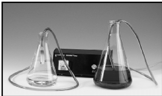
Figure B. Adsorbing Ethidium Bromide on Rezorian A161 Cartridges — Pump Method
