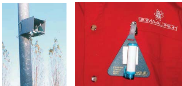
Figure 3. Outdoor (left) and personal (right) sampling. Outdoor sampling using the radiello shelter. The sampler consists of the diffusive body (white cylinder), the adsorbent tube (not shown, inside the diffusion body), and the blue triangular support plate.
