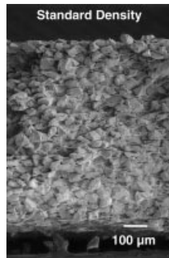
Micrograph of a cross section of a standard density (SD) Empore disk (40-60 µm particle size)
