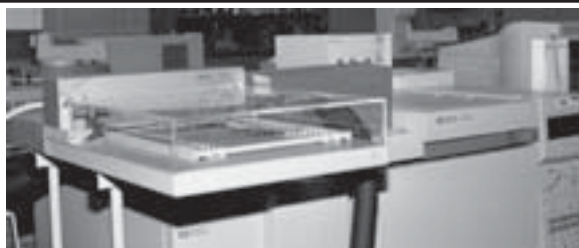
Figure 1. GERSTEL TDS A Coupled to a HP6890GC/5973MSD
