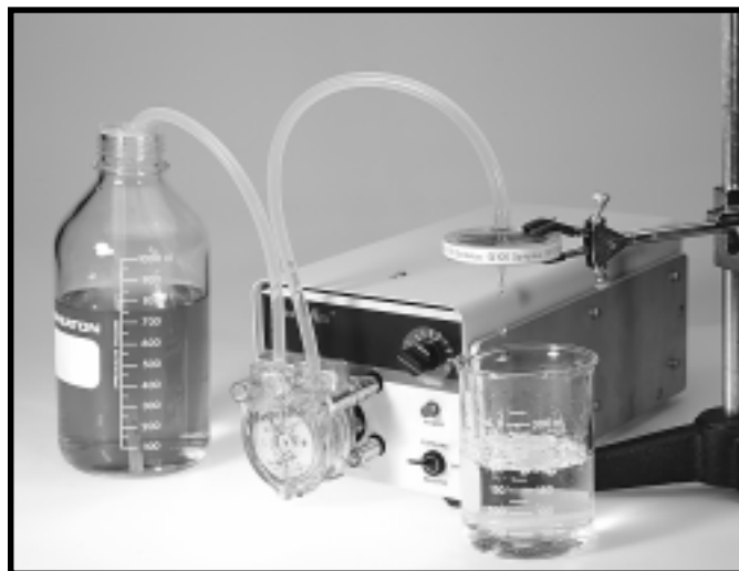
Figure G. Sartobind Membrane Adsorber Unit Connected to a Peristaltic Pump
