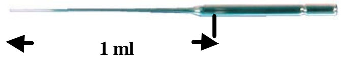
Figure 2. Illustration of a Pasteur Pipette with a Mark Indicating a 1 ml Volume.
