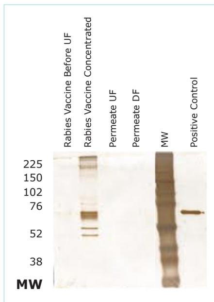
**Figure 6.** Silver staining analysis of samples following ultrafiltration and diafiltration.
