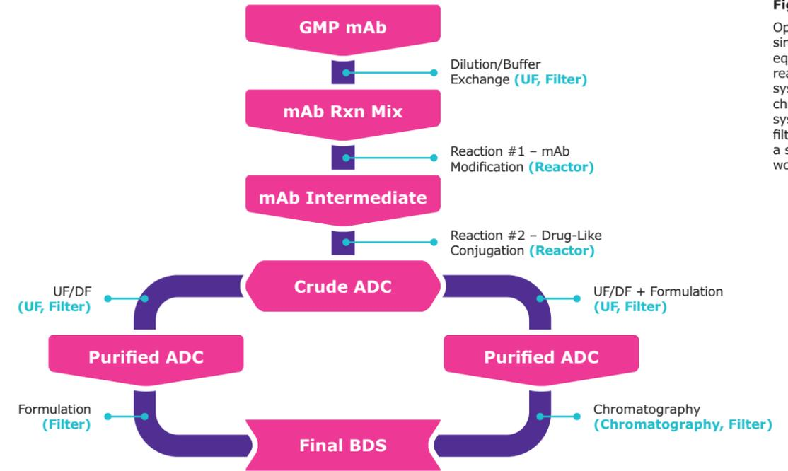
**Figure 2:** Opportunities for single-use equipment – such as reactors, ultrafiltration systems, chromatography systems, and filters – within a standard ADC workflow
