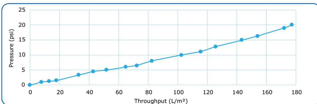
**Figure 3.** Millistak+® HC C0HC pressure profile.
