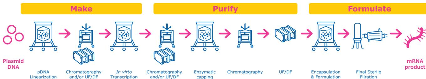
**Figure 9:** General process overview for mRNA manufacturing
