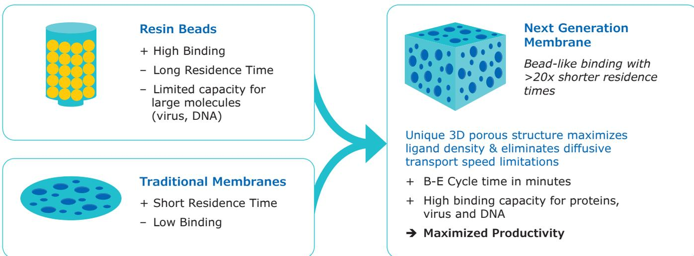
**Figure 3.** Matrix<sup>®</sup> chromatography membrane combines the high binding of resin beads and short residence time of conventional membrane adsorbers.
