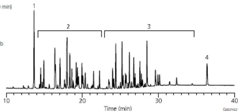
**Figure C.** Aroclors 1016 and 1260 on the Equity-5, 30m x 0.25mm ID, 0.25µm
