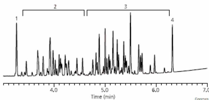
**Figure D.** Aroclors 1016 and 1260 on the Equity-5, 15m x 0.10mm ID, 0.10µm
