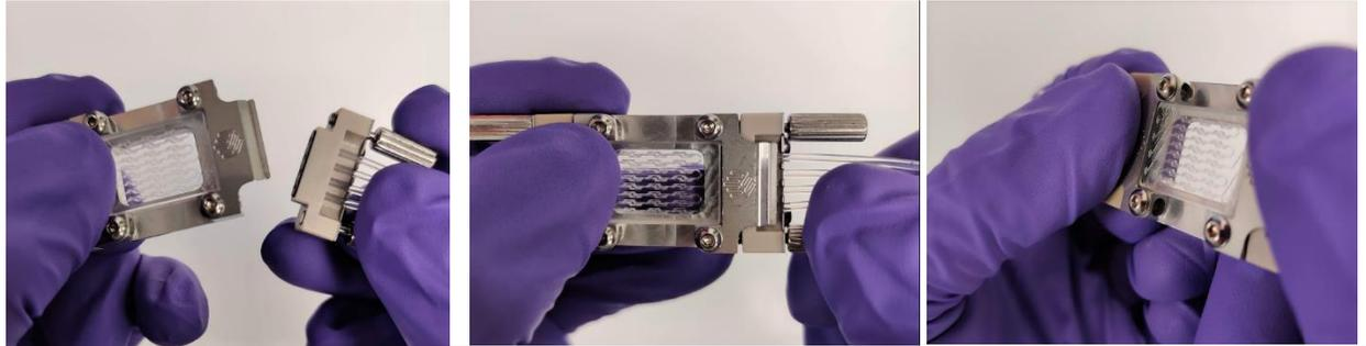
Figure 3: Input line connector and H-interface with chip (left), hand tighten the two screws on input and output connector (middle) and correct alignment between chip and linear connector gasket (right)
