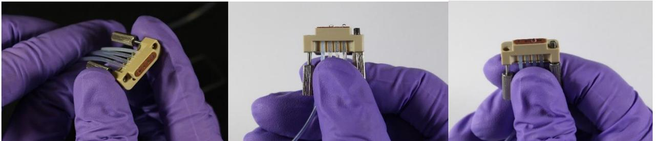
Figure 2: Linear connector (left), droplets of priming fluid forming at the gasket for channel 2 and 4 (middle) and droplet formation for channel 3 (right)
