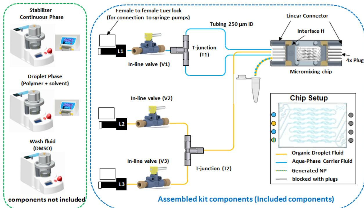
Figure 1: Schematic representation of device kit assembled with the pumps and chip
