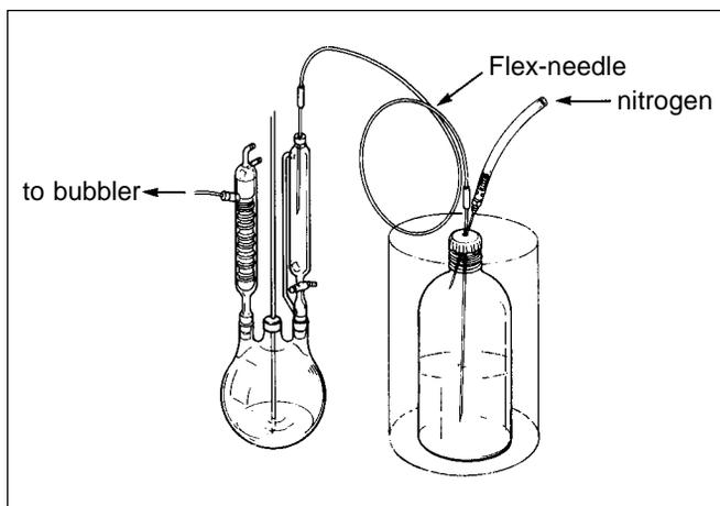
Fig. 2 Double-tipped needle transfer of pyrophoric liquid.
