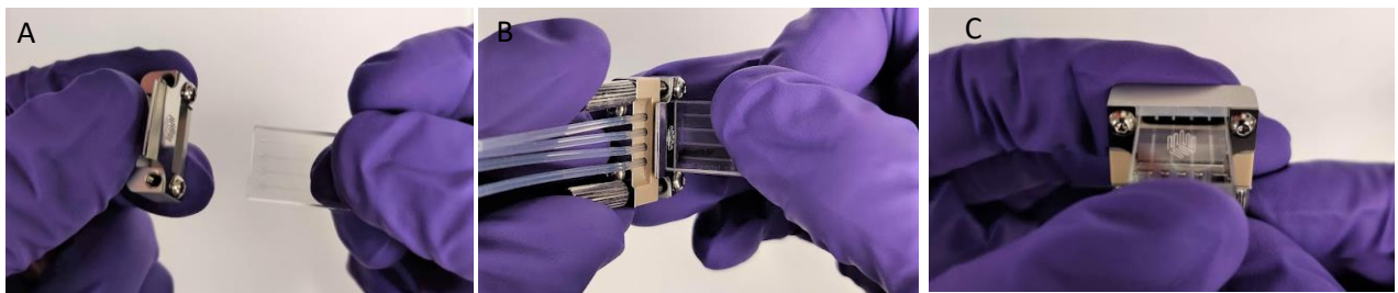
Figure 4: (A) Linear connector preassembled with top interface and microfluidic chip, (B) place microfluidic chip at a 90-degree angle to the top interface and hand tighten the two screws on the linear connector, (C) correct alignment between chip and linear connector gasket
