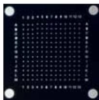
**Figure 1** Image of the single cell micro-array square of 13 x 13 spots. Each spot has a diameter of 100 μm. Two arrays are placed on an omniphobic coated ITO slide in dimensions of a standard microscope slide.
