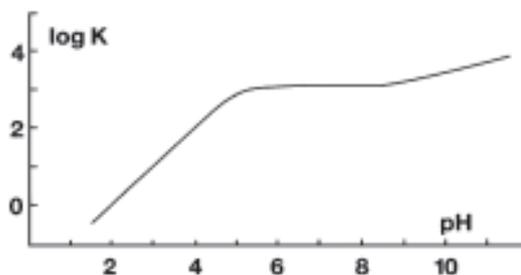
**Figure 1** Dependence of the reaction rate constant  $K$  on the pH (Verhoef, J.C. and Barendrecht, E.; Mechanism and Reaction Rate of the Karl-Fischer Titration Reaction. J. Electroanal. Chem. 1976, 71, 305–315)
