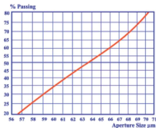
Figure 1 Calibration graph for the 63 µm sieve standard
