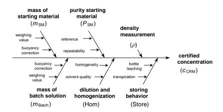
The combined uncertainty  $u_c$  is calculated by combination of the squared contribution values. The expanded uncertainty U is then calculated to a confidence level of 95%, by multiplying  $u_c$  with a confidence level factor of k=2.
