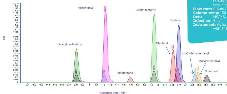
Figure 2: LC/MS/MS results of the analysis of the nine fentanyl analogs on Ascentis Express Biphenyl column
