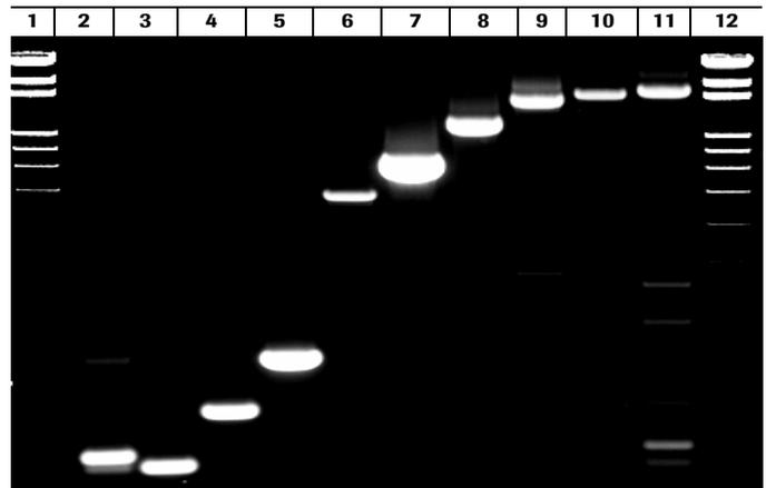
**Fig. 3: Long fragments from a variety of templates.** The Transcriptor One-Step RT-PCR Kit generates fragments up to 6.5 kb. RT-PCR on various fragments from different sources was performed according to the standard RT-PCR protocol. Aliquots of 15  $\mu$ l of each RT-PCR reaction were analyzed on an agarose gel.
