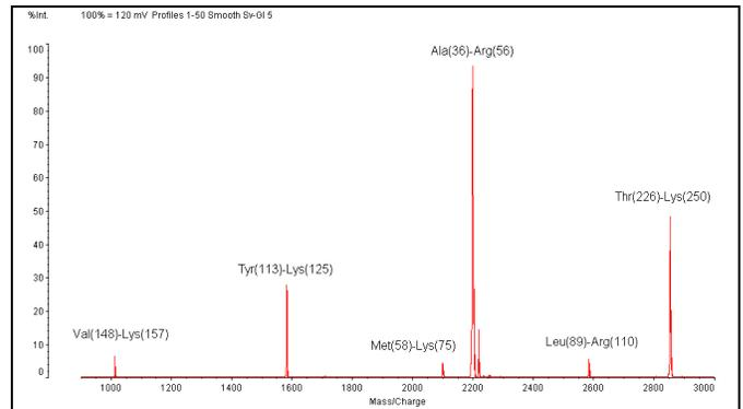
The substrate protein, carbonic anhydrase II (0.5 µg), was separated on a 4–20% Tris-Glycine gel. The spot was removed and digested using the protocol for in-gel digestion. The matrix ( $\alpha$ -cyano-4-hydroxycinnamic acid) was prepared at 10 mg/ml in 70% acetonitrile with 0.1% TFA. The digest solution was desalted using a C<sub>18</sub> ZipTip and 1.5 µl of the matrix solution was used to directly elute the peptides onto the MALDI target.
