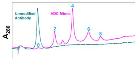
4.6 mm × 10 cm TSKgel butyl-NPR column run at 0.4 mL/min
