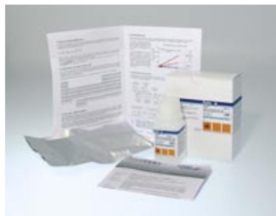
Figure 6 ..... Packaging of TraceCERT™ Ultra standards for ICP to ensure \pm 0.2\% expanded uncertainty for the certified value. Only when using specially selected Al-coated bags the specifications of the CRM can be guaranteed to have a shelf life of up to 4 years
