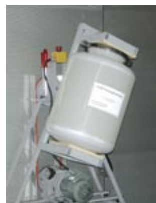
Figure 4 ..... The 60L PVDF containers for overhead tumbling of TraceCERT™ standards guarantee the complete homogenization and ensure that no contamination from container wall into the solution and also no adsorption of analyte on the container wall can occur.
