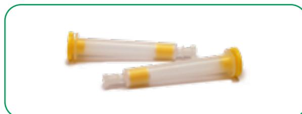
The LpDNPH S10L cartridge is a 3 mL reversible cartridge design for EPA Method TO-11A which is designed for the analyst who prefers shorter dimensions and does not require an adapter for sampling. The cartridge is eluted by connecting to an empty SPE cartridge that acts as a reservoir for gravity-fed elution solvent. The S10L is equivalent to both the Waters Sep-Pak® cartridges and XpoSure™ cartridges.
