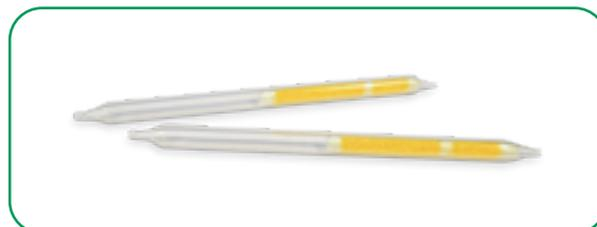
The LpDNPH S10 cartridge is a 3 mL SPE style cartridge with a slip luer design and a built-in reservoir for easy extraction and elution. Reusable adapters are available. The S10 Starter Kit contains all needed adapters (tubing and cartridge adapter).
