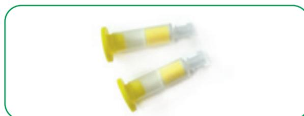
DNPH Rezorian™ cartridge is a 3 mL cartridge which features luer-lock end-fittings that can be used to connect a pump tubing to two cartridges in a series for “piggybacked” sampling to monitor breakthrough or an increased capacity.
