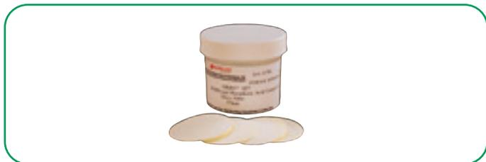
For sampling selected carbonyls where particles are a concern, filter methods are commonly used for compounds such as glutaraldehyde (OSHA 64), crotonaldehyde (OSHA 81), and valeraldehyde (OSHA 85). The glass fiber filters are coated with 2,4-DNPH, actively sampled in a cassette and desorbed in the same manner as a traditional DNPH device.
